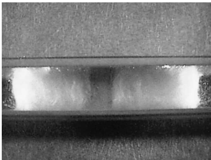
Fig. 2. Photograph of the fine powder catalyst secured in quartz reactor tube. Dimensions of catalyst plug are 2 mm \times 4 mm in diameter.
